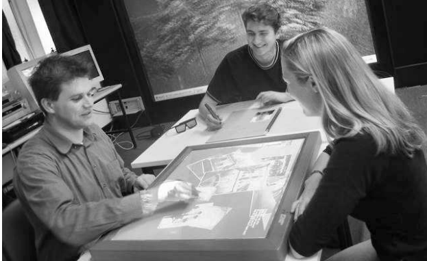
Figure 1. A DiamondTouch in operation, showing the SharePic photo-sharing application
